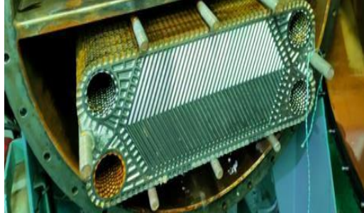
Gambar 2.2 Evaporator Heat Exchanger
