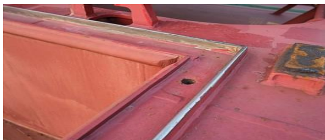
Gambar 0.10 Drain channel dan drain line
