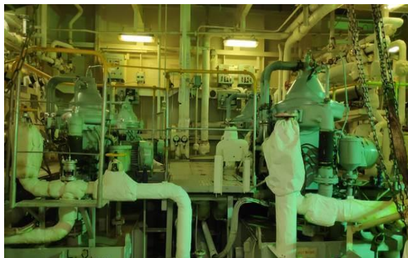
Gambar 2. 1 Purifier di Kapal Sumber : https://shipfever.com/
