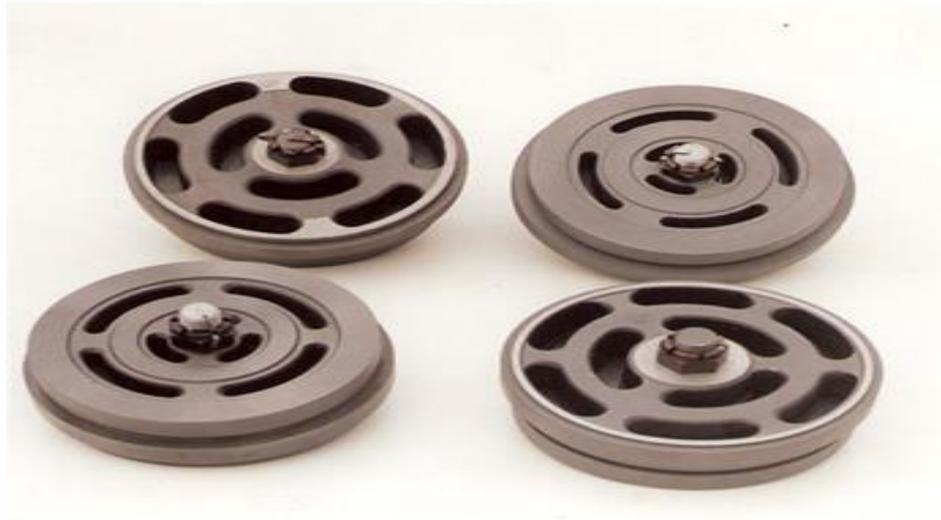
Gambar 3.1 Katub Low pressure and high pressure.
